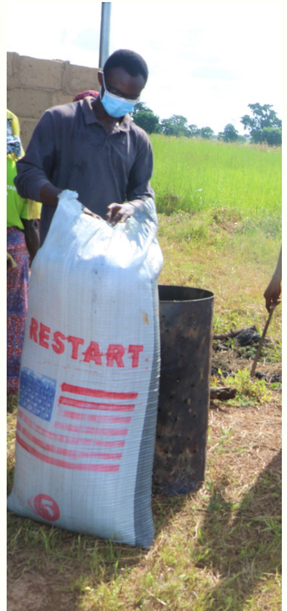
A member of Cletus Team using the metal drum to char the rice husks.
